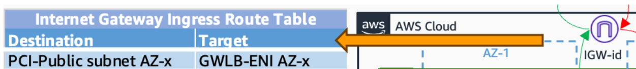
Figure 14: Internet Gateway ingress route table
