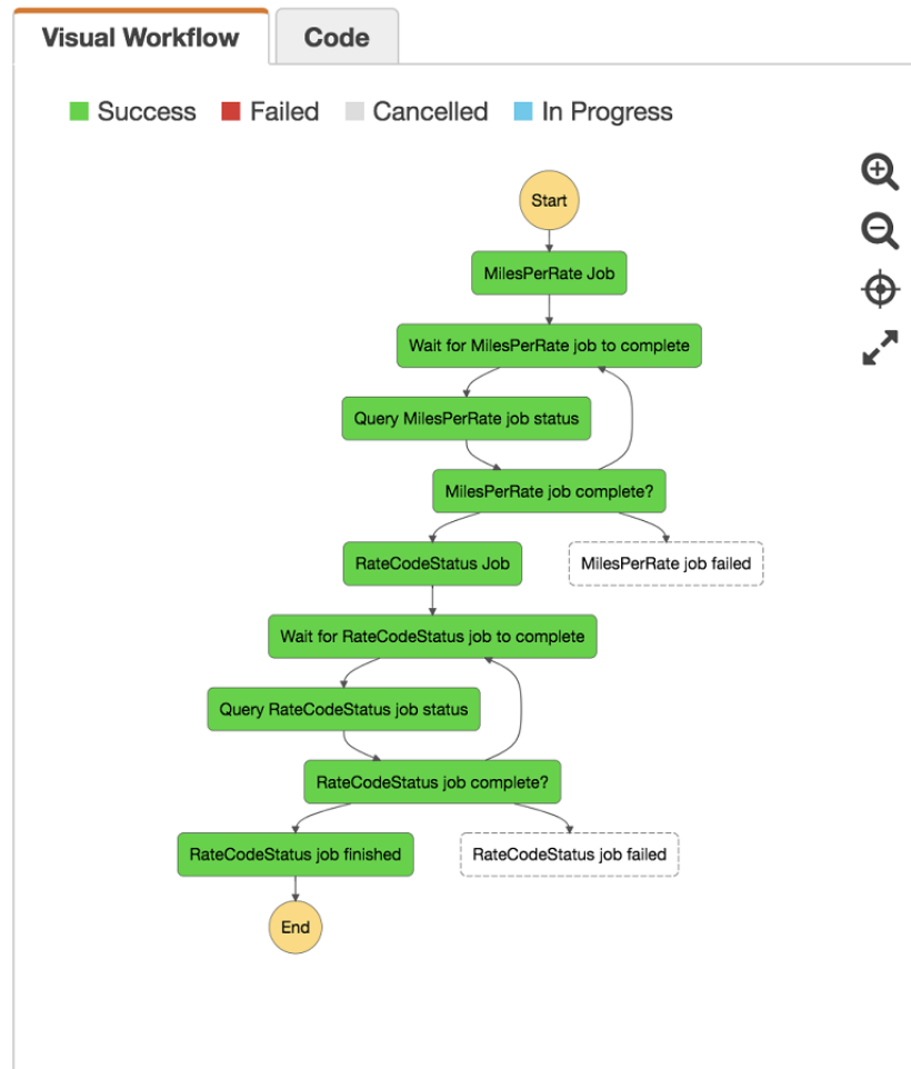
Figure 41: Multiple Apache Spark jobs orchestrated with AWS Step Functions
