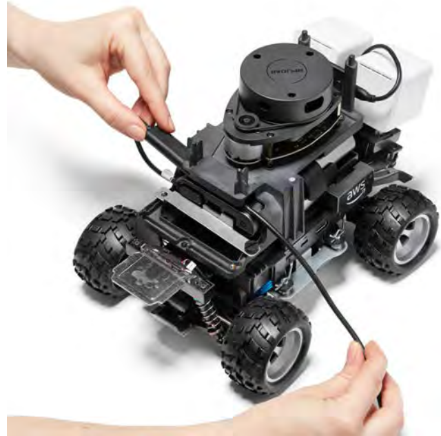
2. Slide cable under LiDAR frame
