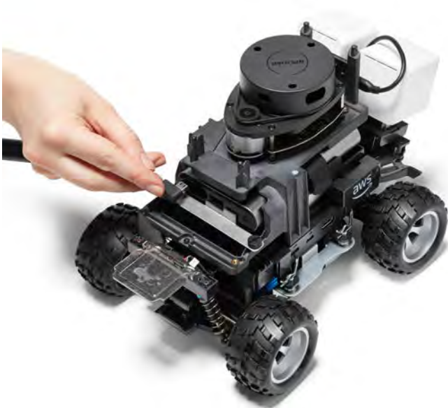
1. Plug cable in Dell compute battery
