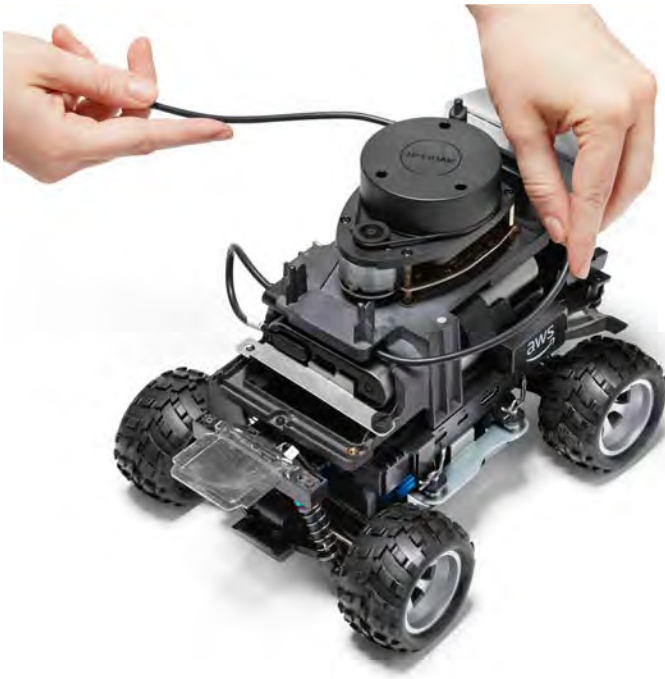
1. Plug cable in Dell compute battery
