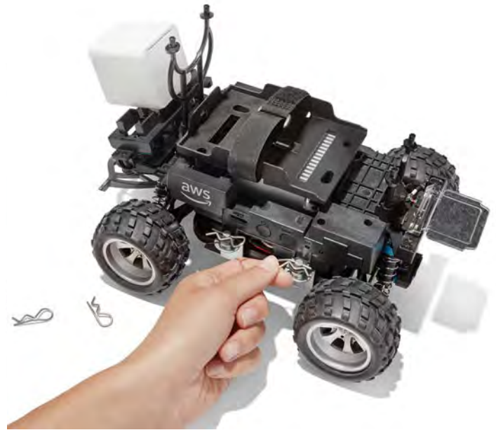
2. Unpin chassis by removing four pins
