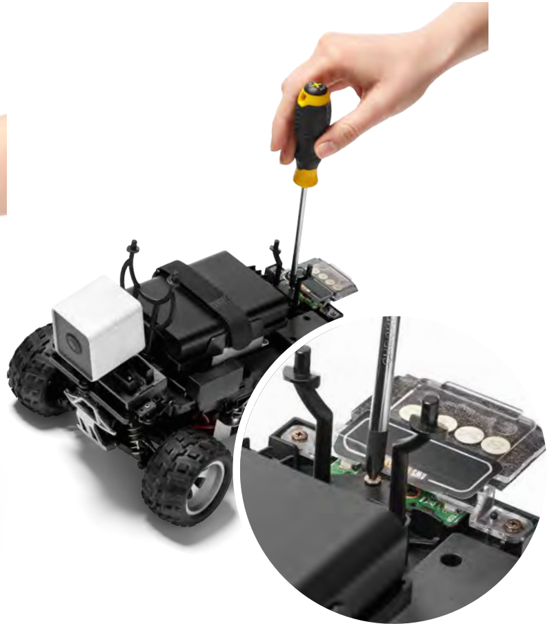
2. Unscrew shell brackets
