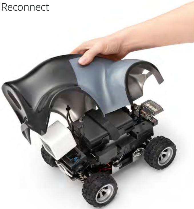
1. Unpin and remove shell
